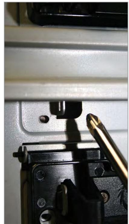
We had to insert our screwdriver into holes such as this to secure our new drive in its bay.
