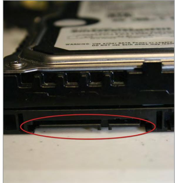
The rear edge of this hard drive shows its L-shaped SATA connectors. The power connection is the longer one on the left.
