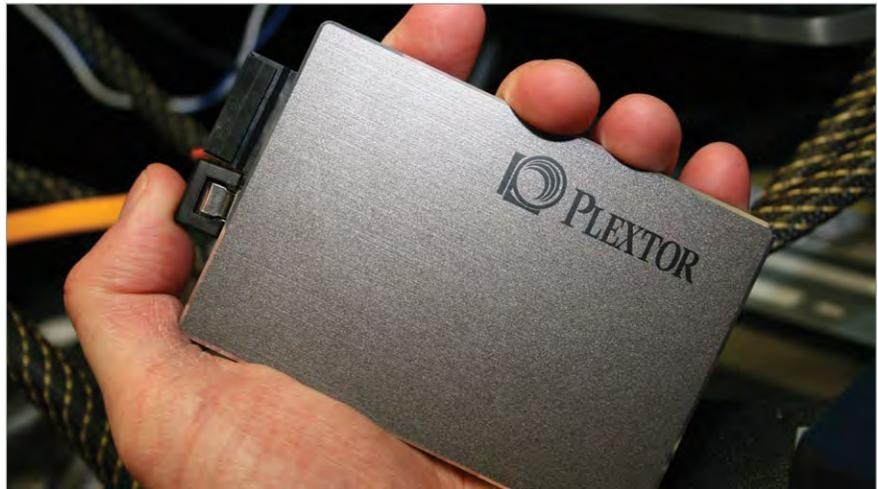
Like notebook hard drives, 2.5-inch SSDs such as this Plextor have different mounting hole patterns than 3.5-inch drives. Since SSDs started to gain popularity, however, some newer cases started to include mounting holes for the smaller drives.
